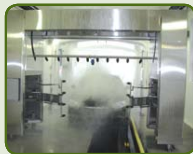
SoftLine's High-Pressure Arch with top and side booms extended to clean the grill area as the car approaches.
